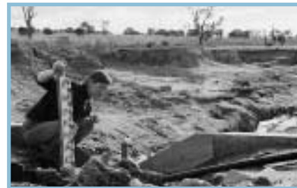
Julie Andrew measures water flow at a V-notch weir on one of the catchments.
