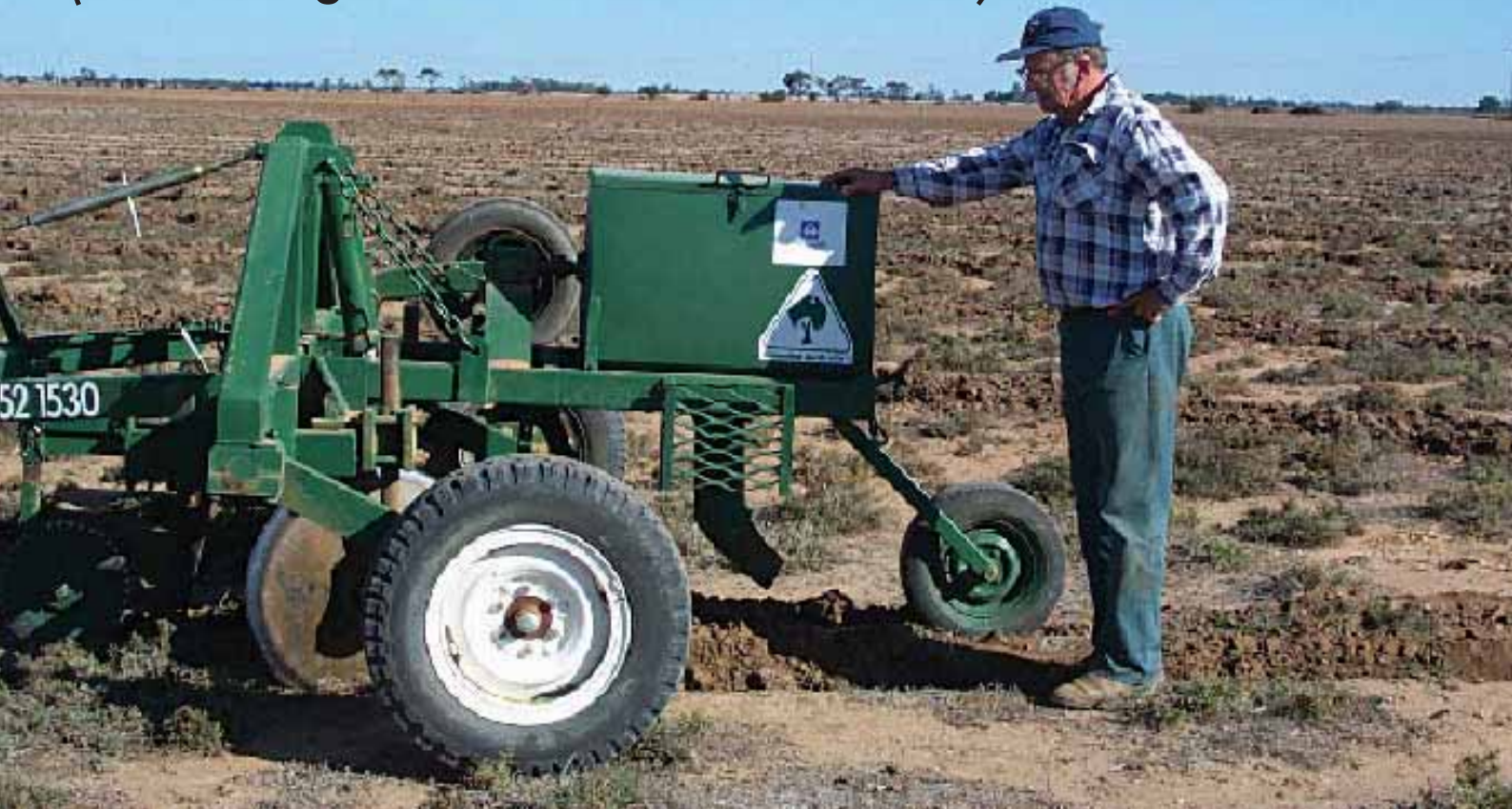
Rod Arnold of Mystic Park with a specialised mounding seeder for saline and/or waterlogged sites. Rod direct seeded 50 acres of saltbush with this machine in 2002.
