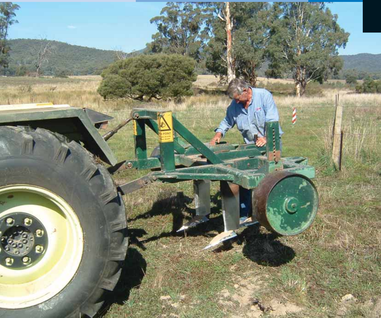
North-east ripping contractor Jack Frewin adjusts his three tined ripper.
