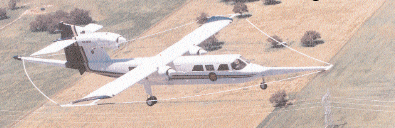
World Geoscience Corporation's Britten Norman Trislander aircraft. This aircraft is now fitted with the SALTMAP system developed by World Geoscience and CSIRO for Landcare applications.
